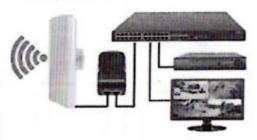
Bridge connects to the POE port of the power supply,the LAN port of the power supply connects to the Switch or NVR Specifications Network bridge dimension: 250\*95\*65mm Finished product dimension: 316\*190\*74mm Net weight of network bridge: 0.3kg Finished weight : 1.0kg
