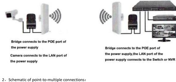
Bridge connects to the POE port of the power supply Camera connects to the LAN port of the power supply Launch angle 60°
