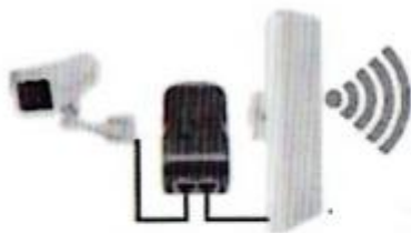
Bridge connects to the POE port of the power supply Camera connects to the LAN port of the power supply
