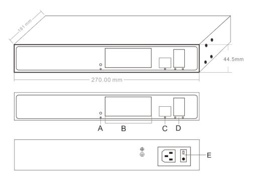
A. Working indicator B. 8\*10/100/1000M RJ45 ports
